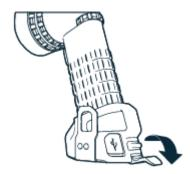
BATTERY COVER To remove the battery, unlatch the Battery Cover. BATTERY This unit has two battery compartments. The Main Battery Compartment (Compartment 1) is located towards the back of the unit. The Spare Battery Compartment (Compartment 2) is located on the trigger side of the unit. Before operation, move the battery from Compartment 2 to Compartment 1.
