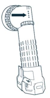
Press the trigger button while Mode Select Dial is in the **Off** position to show battery life.
