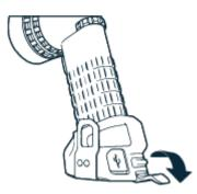
To remove the battery, unlatch the battery cover. After removing the spacer, insert the battery positive (+) side first.
